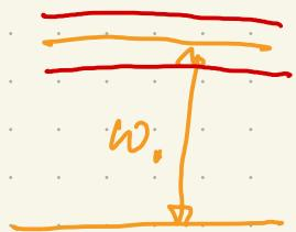
$$\begin{aligned}\dot{\tilde{c}}_e &= -i\omega_e \tilde{c}_e - i \frac{\Omega_R}{2} \tilde{c}_g \\ \dot{\tilde{c}}_g &= -i\omega_g \tilde{c}_g - i \frac{\Omega_R}{2} \tilde{c}_e\end{aligned}$$
